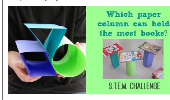
We are going to test the strength of paper, folded in differently shaped columns, by piling books on top. This is very similar to how columns are used to support buildings and other structures. All you need to do is make a circular, square and triangular column. Start balancing books one by one on top and see which one holds the most. The one that holds the most is the strongest!
